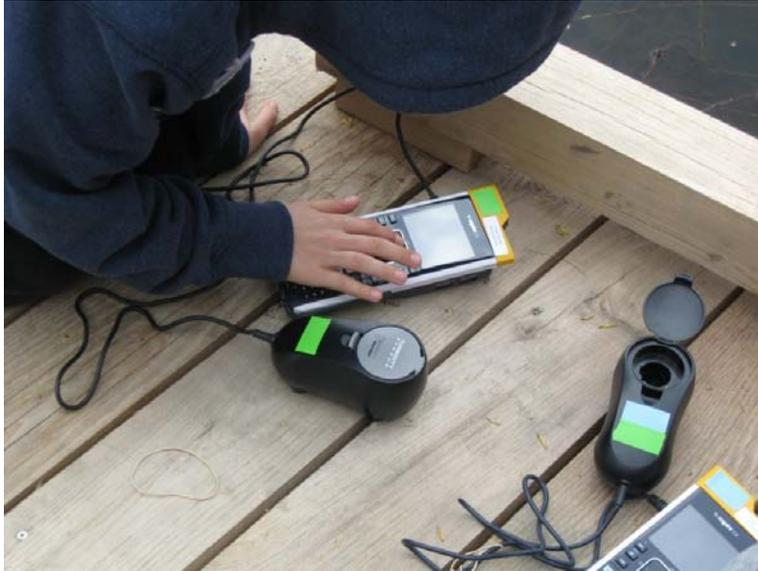
**Figure 11. Collecting water quality data on turbidity using digital probes.**
