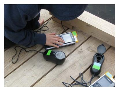
Figure 11. Collecting water quality data on turbidity using digital probes.
