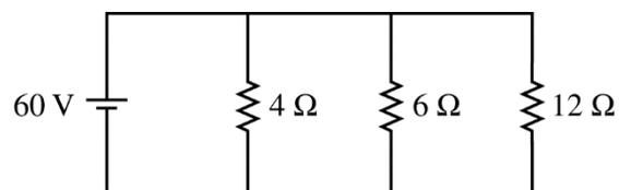
30. What is the equivalent resistance of the resistors in the circuit represented by the preceding diagram?
